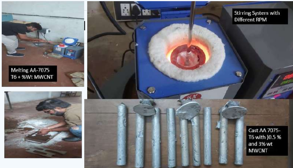
Figure 10 Experiment and preparing the AMMC.
