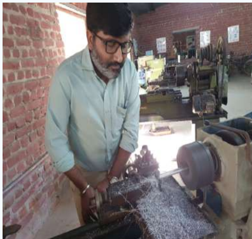
Figure 11 Preparing the specimen as per ASTM E8 for UTS and hardness test.
