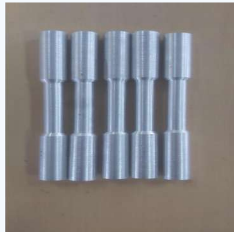
Figure 11 Preparing the specimen as per ASTM E8 for UTS and hardness test.
